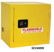
Including 6 Gallon). Powder coat finish. These cabinets feature 14 gauge outside wall construction, lockable flush paddle handle and 4" heavy-duty welded hinges with brass pins. Justrite cabinets include full length piano hinge doors and recessed pad-lockable handle. Self-Close Door models will close via a fusible link that melts at 165° releasing the closing mechanism.
