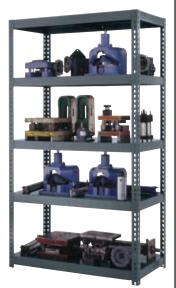
Extra strength boltless shelving units withstand dies, fixtures, jigs and other heavy material. Made using heavy duty steel with a powder coat finish. 16 gauge steel shelves are reinforced with 14 gauge double rivet steel beams for maximum strength. Includes 5 height adjustable shelves that adjust at  $1^{1/2^{\prime\prime}}$  increments. 14-gauge formed angle uprights provide strength and rigidity. Boltless shelving is easy to assemble without the use of nuts, bolts or tools.
