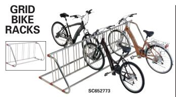
Riveted grid design secures bicycles in upright position. Powder coated galvanized, industrial grade steel withstands years of outdoor use. Framing uses 15/8" dia. tubular steel; grids are 3/4" dia. steel. Double-Sided accommodates bikes on either side. 3 anchor styles: Cement for use in fresh concrete or asphalt, Earth for soil and lawns or 6" Spikes for permanent mounting in existing pavement. Easy assembly.
