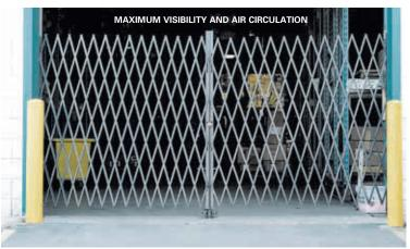
Constructed of strong 3/4" 14 gauge steel channel. Exclusive design protects the durable gray powder coat finish from scratching when folded for a longer life. Assembled with non-corroding zinc-plated rivets. Includes smooth rolling wheel and padlock lug. Double Gates have a cane bolt that holds left half in position and both halves open fully. **Gates fold completely and swing 180**° for unobstructed access. Gates can be either recess or surface mounted. Easy to install.
