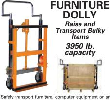
Safely transport furniture, computer equipment or any odd-shaped item easily. Simple hand-operated hydraulic jack raises and lowers loads at controlled speeds. 23"W x 21/4"D lift plate raises load to 10"H. Positive ratchet mechanism with 16' nylon strap secures load. Rolls smoothly on 6" polyurethane casters. 261/2"L x 16"W x 42"H overall and weigh 95 lbs. each. Sold in pairs.
