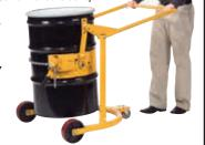
DRUM PALLETIZER Moves and transports drums easily to or from pallets with a maximum height of 8". Dual ratchet stops hold the weight of the drum, and provide several positions where the handle stays until operator takes hold. Operator holds no weight and does not need to balance drum truck. Two 6" polyolefin load wheels and two 4" swivel casters provide smooth movement. Designed for rimmed 55-gallon steel drums.
