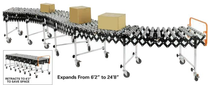
Instantly set-up conveyor lines for shipping, receiving, assembly and packaging areas. Flexible, portable gravity conveyor expands from 6'2" to 24'8". Rugged <sup>5</sup>/16" steel axles and self-tracking skate wheels with enclosed steel ball bearing offers smooth material flow. 175 lbs. per foot capacity. 11/4" (compressed) to 4" (expanded) axle centers for 7" minimum package size. Seven zinc
