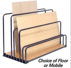
Stores sheet materials. Includes 3 pairs of  $1^3/16^{\circ}$  dia. steel pipe uprights at 12", 26" and 36" heights steel framed wooden deck with lacquer finish.  $1^1/2^{\circ}$ H  $x^{1/2}$ " thick angle iron frame has rounded safety edges. Provisions included for floor anchoring. Blue enamel finish. Frame sockets permit 31/2" upright adjustments (24"W has 7 sockets; 30"W has 9 sockets). Mobile Rack has 6" mold-on rubber wheels and 2,000 lb. capacity.
