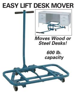
Quickly move a double pedestal desk without removing contents or drawers. Positive safety latch automatically locks in the raised position. Heavy duty 2" rubber wheel swivel casters rotate 360° for easy maneuvering. Overall size - 22" x 32". Height 9³/4" raised, 5¹/2" lowered. Removable handle and tubular lift frame assembly is completely coated with nonmarring material. Chip resistant blue finish.
