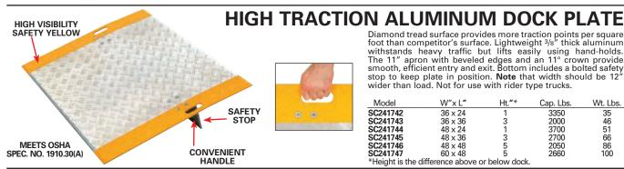
Diamond tread surface provides more traction points per square foot than competitor's surface. Lightweight 3/8" thick aluminum withstands heavy traffic but lifts easily using hand-holds. The 11" apron with beveled edges and an 11° crown provide smooth, efficient entry and exit. Bottom includes a bolted safety stop to keep plate in position. Note that width should be 12 wider than load. Not for use with rider type trucks.
