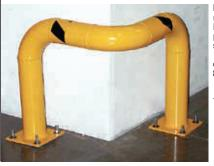
Fits snug around corners to protect machinery, buildings and offices. Heavy duty welded steel with yellow powder coat finish and 3"W black stripes. Constructed of 4" schedule 10 steel pipe with 41/2" outer diameter. Base plates measure 8" x 8" and allow floor anchoring.
