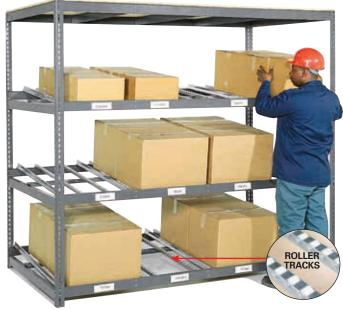
Provides first-in-first-out rotation. Roller tracks have U-shaped galvanized steel channel sides with plastic wheels that support 50 lbs./ft. Guide rails and beams adjust to accommodate carton sizes. Each level includes 4 pairs of roller tracks, 5 guide rails and 1 cross support. 5/8" thick particle board top shelf supports 1000 lbs. of storage. Levels adjust on 11/2" centers. Gray baked enamel finish. Easy assembly.
